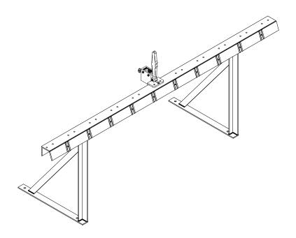
For use with tee and jay bar guides and Series 70 tension blocks. The locking rail is provided with a continuous index card strip and card holders for set identification. Standard set spacing is 6", 8" 9" and 12" on center. Please specify with ordering.
