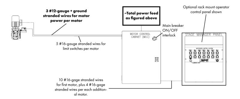
Ex: 4 motor system would have 22 #16-gage wires.
